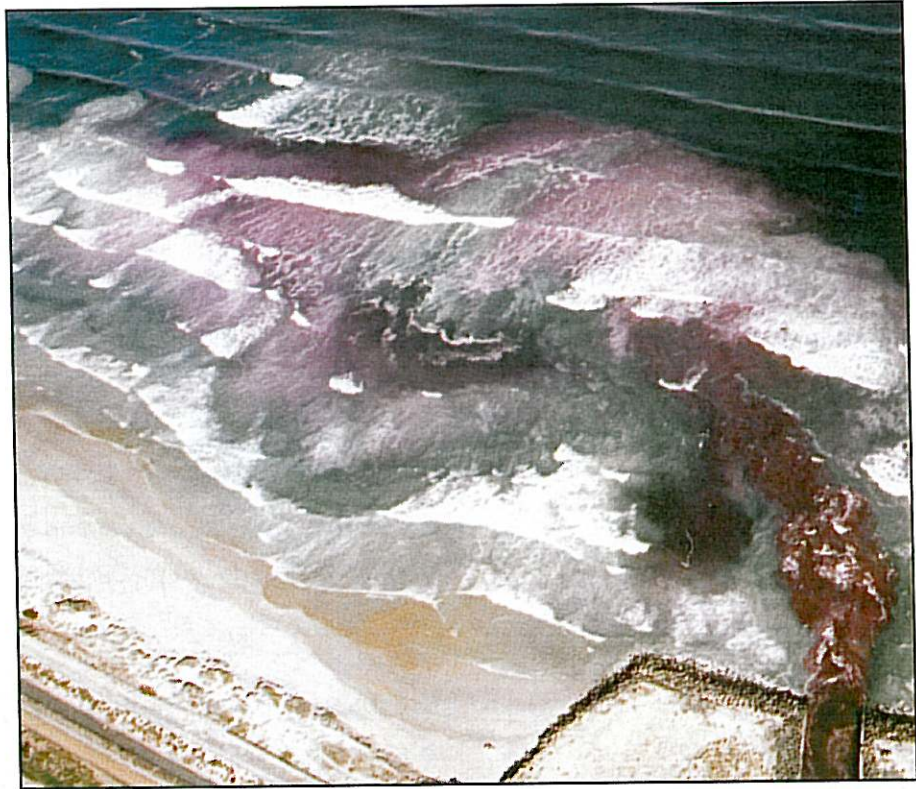
Test to determine the dilution of liquid effluent discharged from Koeberg power station
