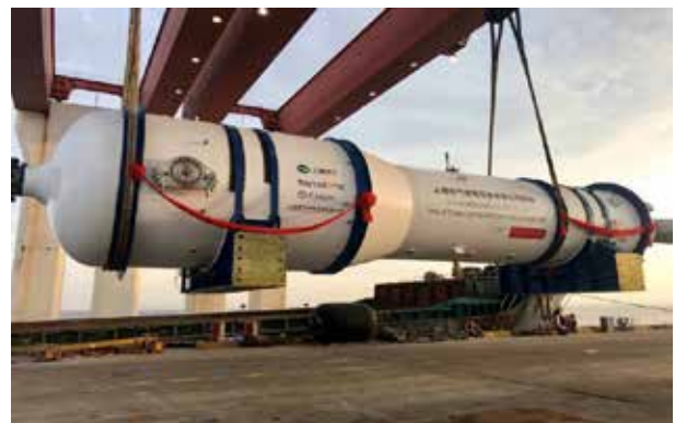
Figure 4: Replacement steam generators being loaded for shipment to South Africa
