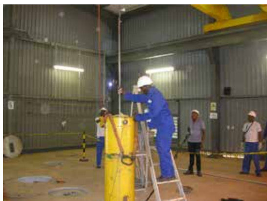
Figure 10: Storage of Used Fuel in Thabana Pipe Storage Facility using the approved Cask
