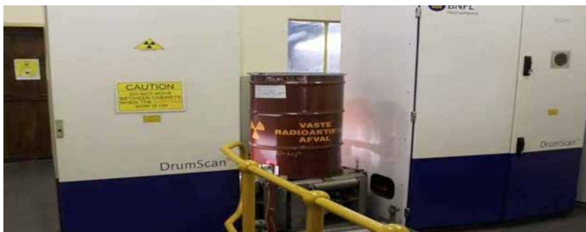
Figure 29: Drum going through the Segmented Drum Scanner at Bus Shed
