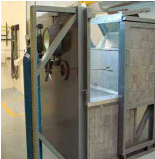
Figure 30: Lead shielded cell for source conditioning
