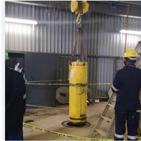
Figure 12: The transport cask being placed over SAFARI-1 storage pipe
