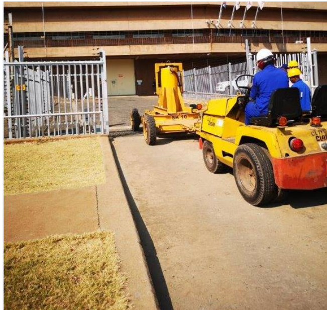
Figure 13: Cask being transported between SAFARI-1 and the TPS.
