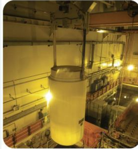
Loading of spent fuel casks.
