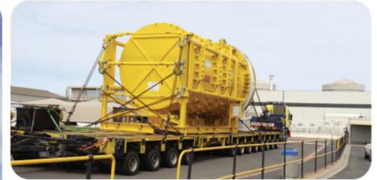
Arrival of the Reactor Pressure Vessel Head and Control Rod Drive Mechanisms at Koeberg.
