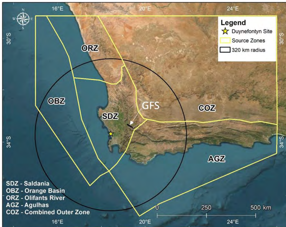
Figure ES-3. Seismic source zones defined in the SSM for the Dwynefontyn PSHA.
