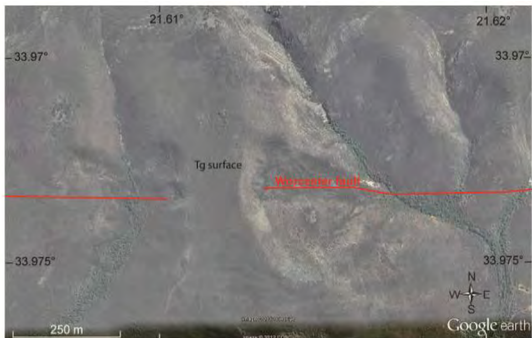
Figure 8-64. Google Earth image showing unfaulted geomorphic surface (pediment or eroded pediment) across the mapped trace of the Worcester Fault (Bommer et al., 2013). Tg- Grahamstown Formation.
