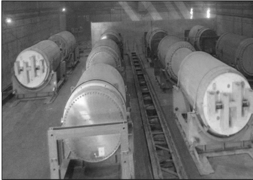
Umfanekiso 23: Imigqomo yokugcina amafutha ekufakwa kuyo ii-assembly zamafutha enyukliya
