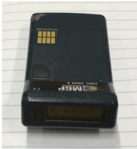
Figure 11: Electronic personal dosimeter (EPD) [61]
