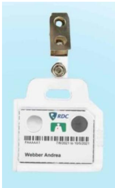
Umfanekiso 12: I-Thermo-luminescent dosimeter (TLD) [62]
