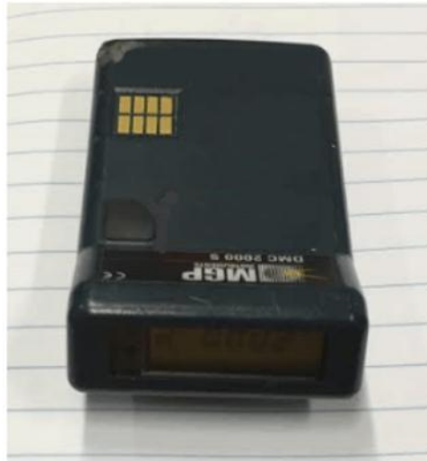
Umfanekiso 11: Idosimitha yomntu ngamnye ye-elektroniki (i-EPD) [61]
